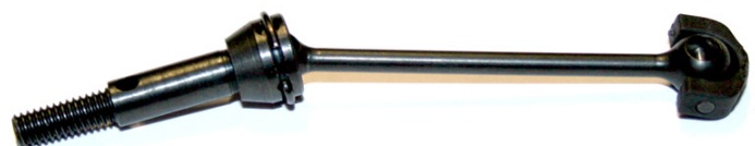
Step 4: Job is done ! G-clip well positioned
