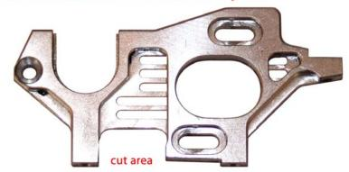
To obtain more flex on the rear of the car, I modified my motor mount to obtain less contact between the chassis and the aluminium part.
