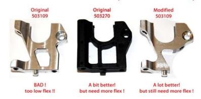
With the original 503109 part, the car is too hard, due to the lack of flex. We tried to run without the 503106 linkage post, it goes really better, but the chassis don't will appreciate for long. We also tried with the 503270 plastic version, it is a bit better but not sufficient. So, I cut the 503109 part with my Dremel; it's a lot better - really better.
