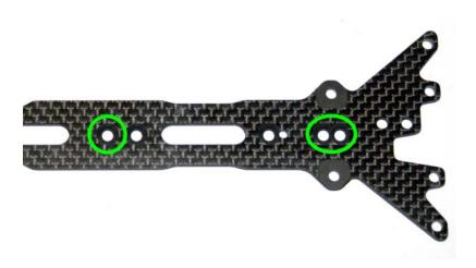
I modified my upper deck to only use flat head screws. This modification allow me to use big lipos on my car, without damage the lipo's plastic case.
